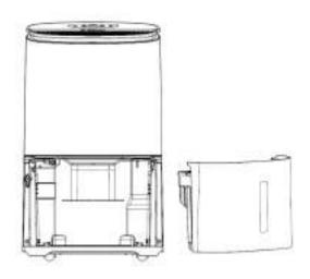
Step 1: Remove the water tank.
