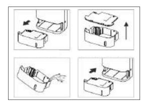
The dehumidifier has a built-in tank, which the water will automatically drip into. When the tank is full, the dehumidifier will switch off and the light for the full container will light up. The tank must now be removed, emptied and put back. The dehumidifier will now restart with the same settings it was set with before the tank was full.
