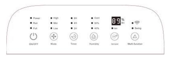
**On and off:**Here the dehumidifier is switched on or off. The correct mode (button 2) and humidity (button 4) must be set. The fan will always be in operation 4 minutes after the dehumidifier is switched off (power lamp lights up red). This is to cool the dehumidifier.
