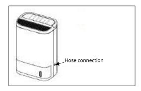
If you want to drain away the water, this can be done via the water outlet. Make sure the hose has a fall all the way down to the drain. If the hose is blocked, bent or going upwards, the water will enter the tank and the dehumidifier will stop when the container is full. If the hose is removed, the water will go into the water tank.
